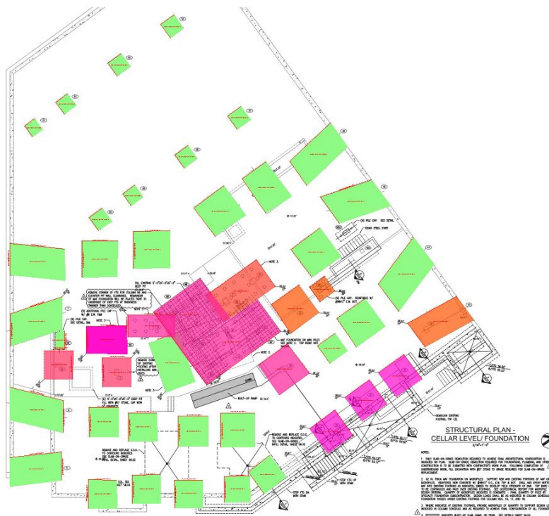
Figure 36 Pile Cap/Footing Quantity Takeoff
