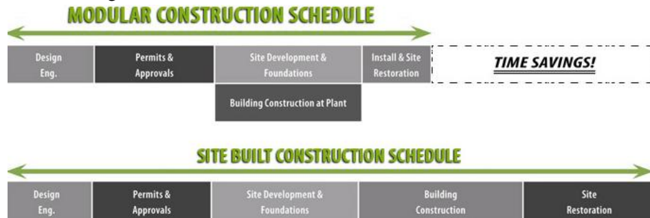
Figure 57 Visual Process Map of Prefabrication vs. Typical Stick-Built Method
