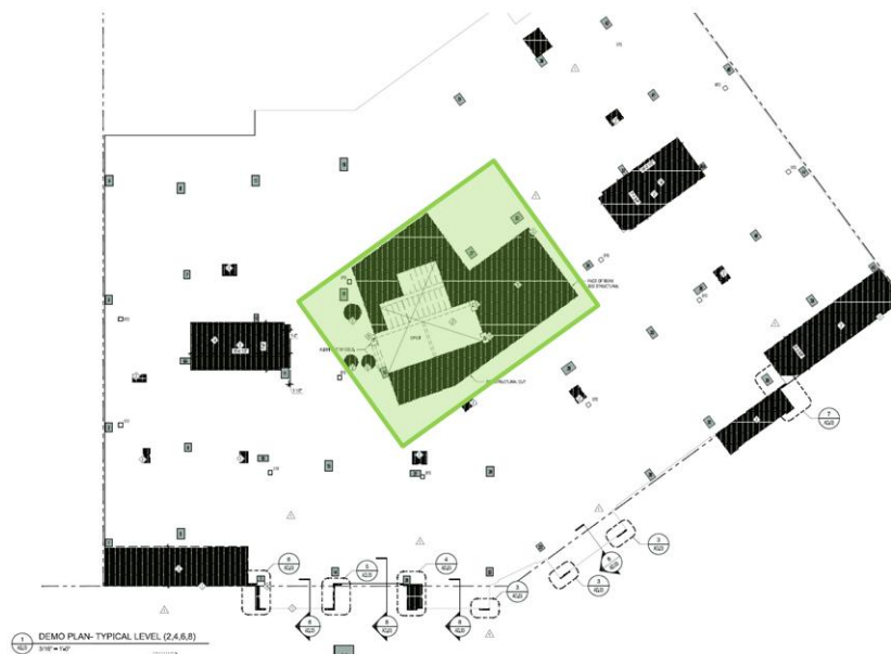
Figure 11 shows the demo plan for the even levels with the typical slab and interior wall demolition
